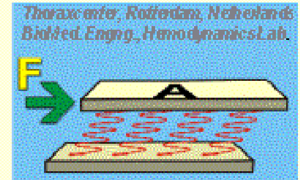
Shear stress is a shearing stress acting tangentially to area A
